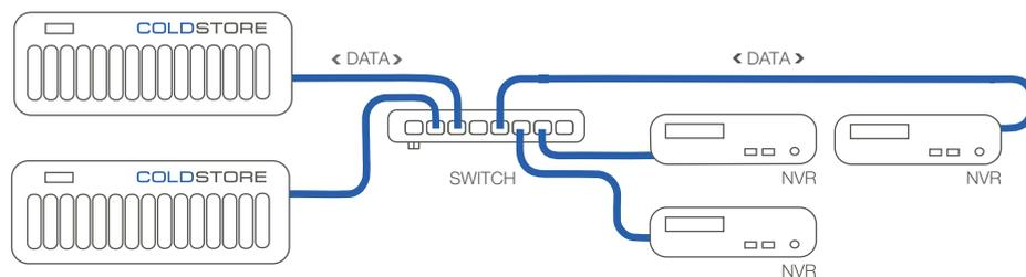
NVRs write to COLDSTORE 3U Pro across the network. Multiple recorders can write to a single COLDSTORE 3U Pro, or one recorder can write to multiple COLDSTORE 3U Pros if required.
