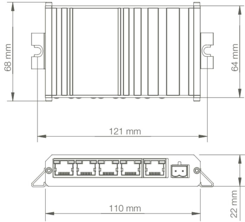
Width 110mm (131mm inc. clips) | Depth 68mm (not inc. connectors)
