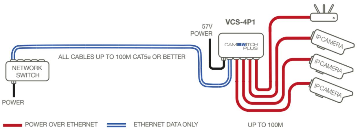
When used with an optional local power supply, CAMSWITCH 4 Plus provides four POE output ports with 15W or 25W per port (802.af or 802.3at).
