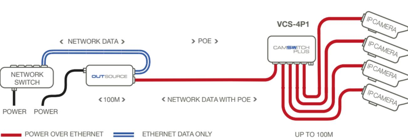
CAMSWITCH 4 Plus can be POE-powered. Veracity's OUTSOURCE injectors and 23AWG Cat6 cables are recommended for POE-forwarding applications.
