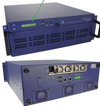
Rear view [above] showing dual Gig-E ports, alarm/relay connections and the dual hot-swap PSU option. Note that the three cooling fans are software controlled and are normally switched off.
