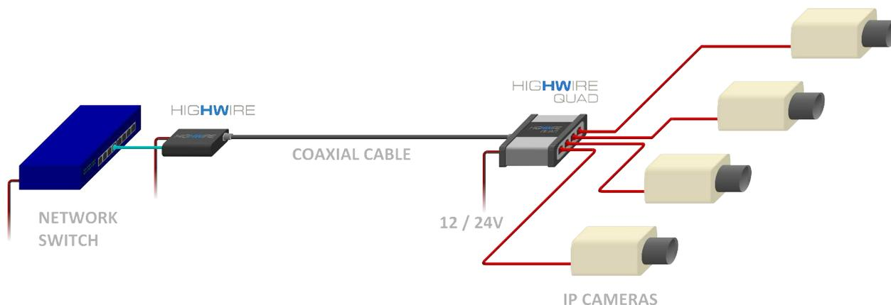
HIGHWIRE QUAD integrates a HIGHWIRE Ethernet-over-coax interface with a four-port 10/100 PoE switch, all powered from a legacy 12 volt DC or 24 volt AC supply. A standard HIGHWIRE at the other end of the coaxial cable is used to convert the signal back to Ethernet.
