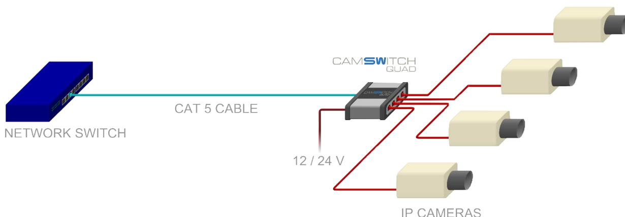
In the example installation shown, CAMSWITCH QUAD allows four IP video cameras to receive their PoE power from a single legacy low-voltage supply.
