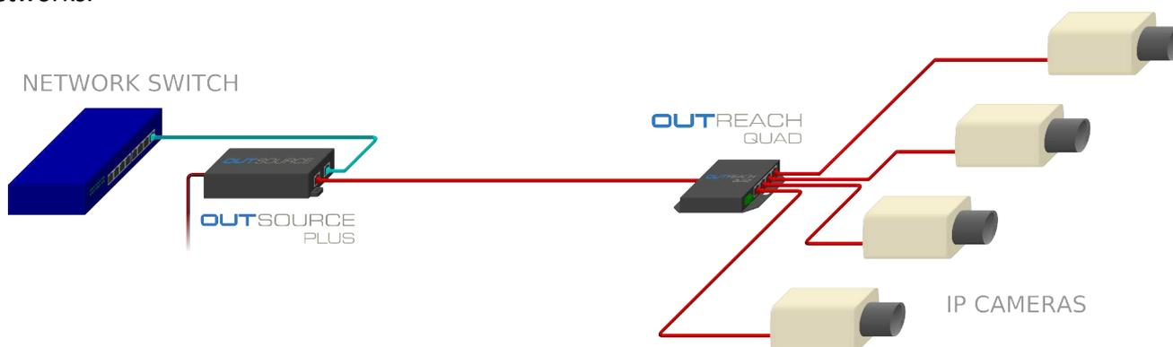
In the typical application shown, OUTREACH QUAD enables up to four IP cameras to draw their power from a single OUTSOURCE PLUS midspan, located up to 200 metres (660 feet) away.
