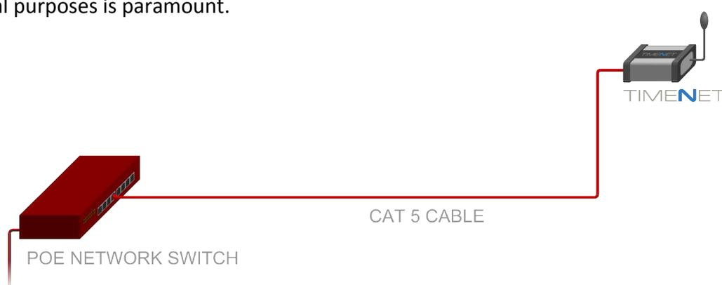
TIMENET is a self-contained NTP master clock and GPS receiver, receiving its accurate atomic time signal via satellite. Its compact dimensions and optional PoE power supply mean it is not confined to an equipment rack, and can be located at the edge of the network, at the optimal site for receiving the satellite signal.
