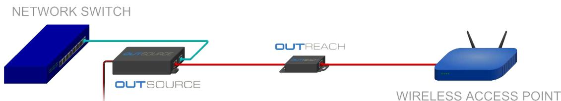
It can also deliver boosted power to OUTREACH for long-distance or high-power applications. In the example above, OUTSOURCE injects PoE power into a standard network switch channel, and provides the extra power required to enable an OUTREACH and a wireless access point of any power class, across 200 metres (660 feet) of cat 5 cable.
