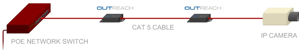
OUTREACH is compact, wall-mountable and self-configuring, and multiple OUTREACHes can be connected in a chain to extend Ethernet connections with or without PoE to up to 1000 metres (3280 feet).
