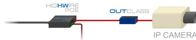
It displays a Class 2 signature as standard, so fitting an OUTCLASS to an unclassified 5 watt IP camera would reduce the power it requested from its PoE source from 15 watts to 7 watts. This allows the power budget of a PoE switch to be allocated effectively. In the above example, OUTCLASS enables operation with HIGHWIRE POE, as HIGHWIRE POE will not deliver PoE to devices that request more than 7 watts.
