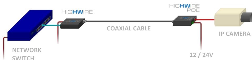
Veracity's HIGHWIRE technology creates an instant 100BASE-T Ethernet connection across up to 270 metres (900 feet) of standard RG-59 cable, so no installation of Cat 5 is necessary. HIGHWIRE POE also converts the existing 12 volt DC or 24 volt AC supply into a universal PoE power source for the new camera.
