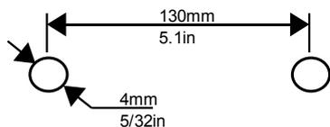
CAMSWITCH QUAD is fitted with two repositionable mounting lugs to allow the unit to be secured to a wall. The recommended mounting hole locations are shown above.
