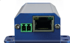
HIGHWIRE Longstar Lite Ethernet and DC input
