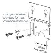
Mounting to flat surfaces: Maximum screw size 3.5mm (#6)
