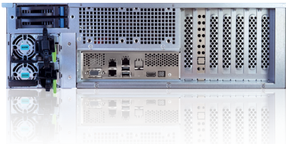
Rear view (above) showing the dual gigabit Ethernet ports, dual hot-swap power supplies and mirrored hot-swap solid state OS disks.
