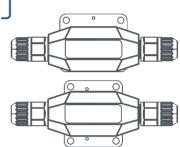
NB Ensure nothing can push on the connectors & that the cables are supported and not in tension. Mount the product horizontally where possible.
