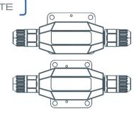
NB Ensure nothing can push on the connectors and that the cables are supported and not in tension. Mount the product horizontally where possible.
