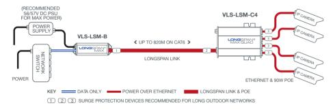
Connect a LONGSPAN Max Base to a LONGSPAN Max Quad and then connect to up to four POE cameras, or other POE devices.
