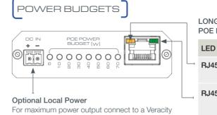
56V-57V power supply only - in polarity shown.
