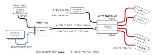
The diagram shows power injection at the Camera end, using a PSU for HIGHWIRE Powerstar Quad, with no power delivery
