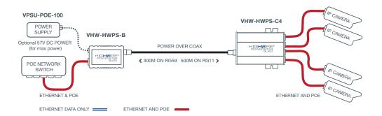
The diagram shows POE power delivery over coax from the Base end. The Powerstar Base device may be powered by a POE or POE Plus switch, or for maximum power delivery over coax, by Veracity's 57V DC PSU. See POE Power Budget Table for POE power outputs.
