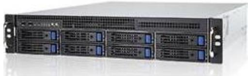
**⚠** Ensure the system has not yet been switched on before mounting the first disks – the COLDSTORE start up procedure requires disks to be present for full boot-up and normal operation. If the system has been switched on in error, simply switch the unit off before proceeding. Note that further disks can be added later while the system is running.
