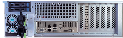
Rear view (above) showing the dual gigabit Ethernet ports, dual hot-swap power supplies and mirrored hot-swap solid-state OS disks.
