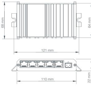
Width 110mm (131mm inc. clips) | Depth 68mm (not inc. connectors) Height 23mm inc. clips | Weight 135g
