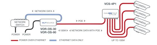
CAMSWITCH 4 Plus can be POE powered. Veracity's OUTSOURCE injectors and 23AWG Cat6 cables are recommended for POE-forwarding applications.
