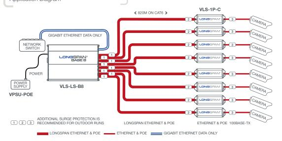
The diagram shows one of many possible configurations for a LONGSPAN Base 8 installation. In this example all channels are
