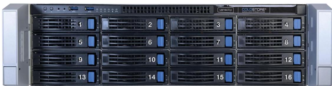
Any make, model or size of SATA hard disk may be used in COLDSTORE. For optimum use of disk space, we recommend that all disks be of identical capacity. Load the disks into the trays using the mounting screws provided.
