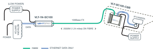
ETHERNET & FIBRE APPLICATION DIAGRAM
