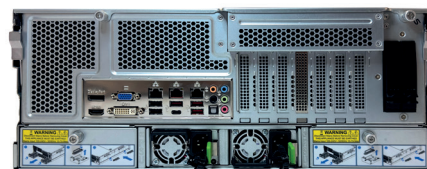
Rear view (above) showing the 1gigabit and 2.5 gigabit Ethernet ports, dual hot-swap power supplies and mirrored hot-swap solid-state OS disks.
