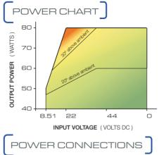
CAMSWITCH 8 Mobile can operate from an 8.5V to 40V DC supply, and steps this up to a steady POE voltage internally.
