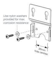
Mounting to flat surfaces: Maximum screw size 3.5mm (#6)
