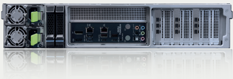
The rear view of VIEWSPAN Plus 9 shows the mirrored, solid-state, 2.5" removable OS drives and the dual hot-swap PSUs. The nine screen outputs are in three rows on the right. Only the two RJ45 network connectors on the main panel are used (1 x Gb, 1 x 10Gb Ethernet)
