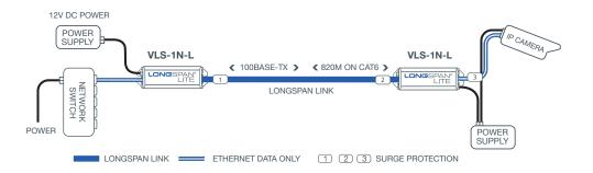
Range is for typical 24AWG Cat5e or 23AWG Cat6, 4-pair UTP. For other cable types, or any installations over 600 metres length, consult Veracity for recommendations or test on site.
