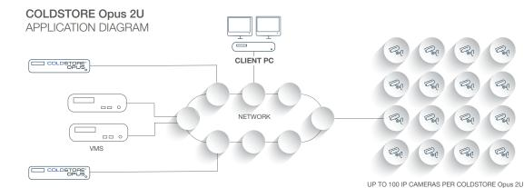
The VMS server writes to COLDSTORE Opus across the network. Multiple servers can write to a single COLDSTORE Opus, or one server can write to multiple COLDSTOREs depending on VMS type. In principle, individual video streams can be routed to any COLDSTORE on the network under the control of specific types of third-party video management systems.
