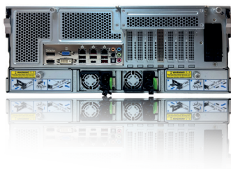
Back view showing dual hotswap power supplies. This robust unit holds 48 disks.
