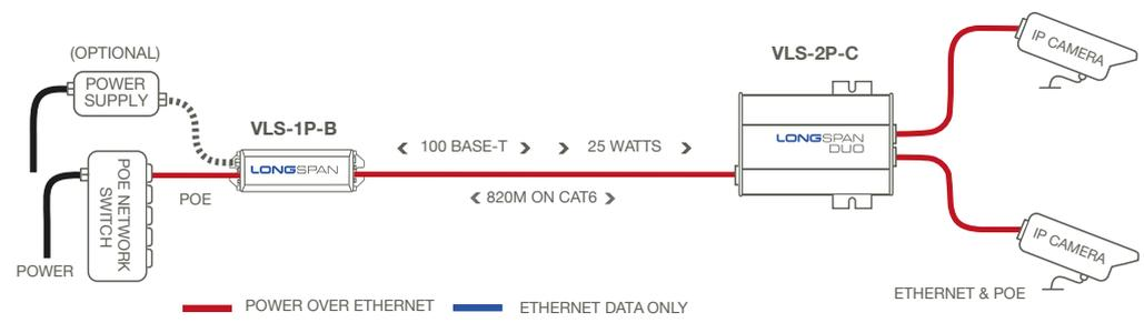
Range is for typical 24AWG Cat5e or 23AWG Cat6, 4-pair UTP.
